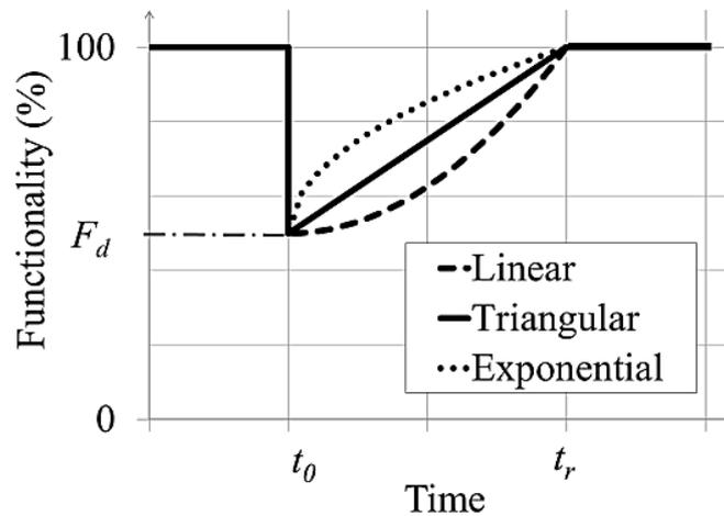
Figure 2 - Recovery functions (adapted after Cimellaro et al (2006, 2010) [2,3,8])
